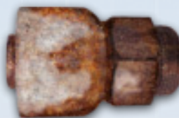
Competitor B after 1,000 hours ASTM B117 (ISO 9227) salt spray test
