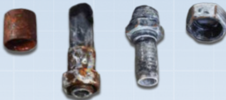
Competitor A after 1,000 hours ASTM B117 (ISO 9227) salt spray test
