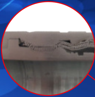
Locking area actively resists axial loading
