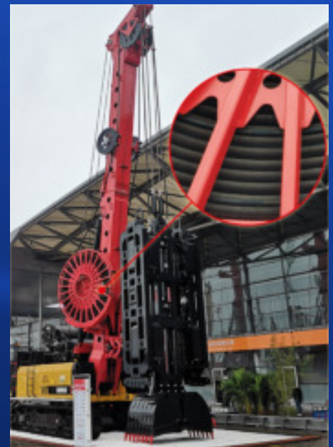
Fig. 7 – HydroRope on hydraulic grab equipment
