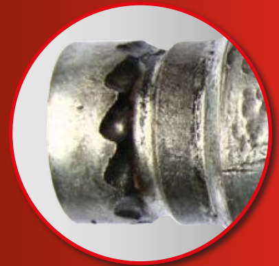
Brinelling on the male coupling
