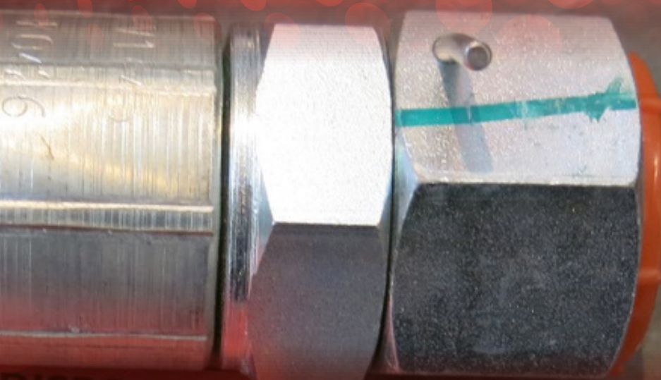
Thrust-wire protruding from termination end
