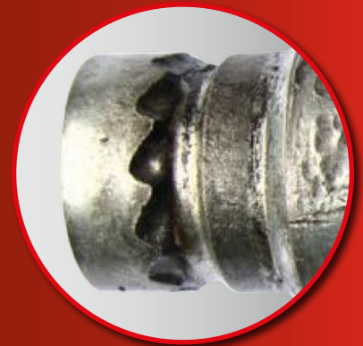
Brinelling on the male coupling
