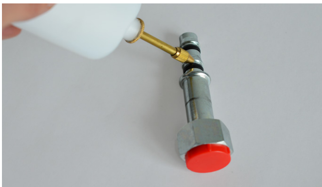
5 Grease the end of the fitting with the same oil used in the air conditioning system
